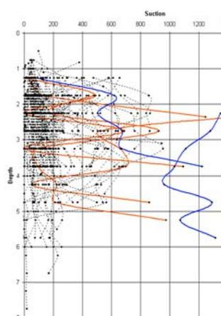
MatLab report a significant improvement in the quality of the filter paper soil suction results since calibrating each batch of filter papers, and are now detecting anomalies prior to issue – see left. The sample consisted of just under 200 tests.
