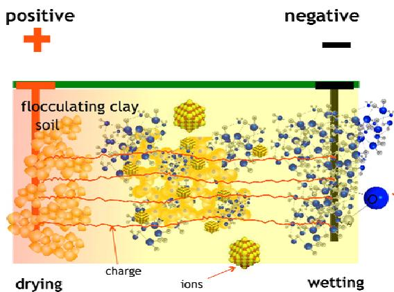
The change is permanent and leads to a reduction in hydraulic conductivity at the positive node. The end-game is to retain the tree, but reduce ground activity beneath the building.
